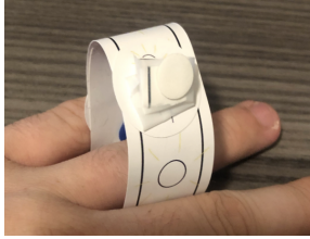
(a) A ring that employs vibration along the inner ring for providing the user with feedback.
